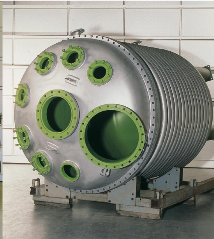
In the spraying sinter procedure (airless and compressed air process), Gutbrod works with Teflon® PTFE and Teflon® FEP. The coating is sprayed on and then „sintered“ at 220°C to 420°C.
